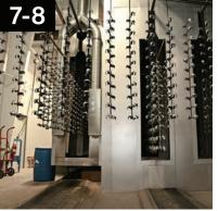
A 200 MPH air blast removes water drops from the pre-treated aluminum. A convection oven completes the dryoff process.
