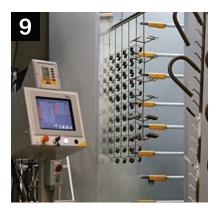
Powder is applied with 18 automated and 2 manual spray guns. Compressed process air is dried to -35°F Dew Point for superior adhesion.
