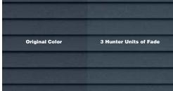
This image is a representation of approximately 3 Hunter Units of fade. Actual fade varies from house to house and is dependent on exposure to weather conditions.
